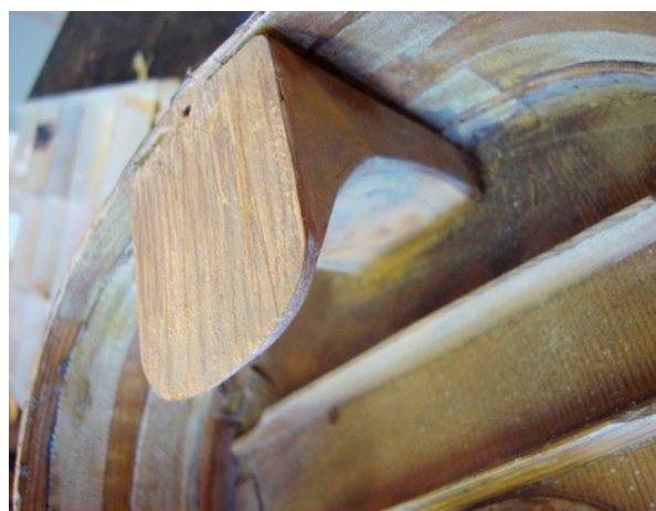
The upper block distant from the ribs, and above on the right, a canvas put "astraddle" style over the ribs and the soundboard.
