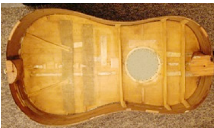
The top has been washed, some positioning cleats are still visible, but marks of twine or linings have disappeared. Purflings and pistagnes are not fixed anymore. (Collection Musée instrumental de Nice – Palais Lascaris)
